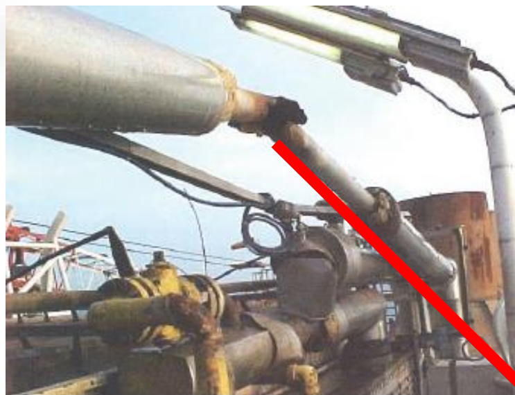
CUI Failure of 4" Gas Compressor Recycle Line
